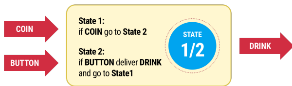
Fig. 2. A Coke Machine expressed as a state machine
